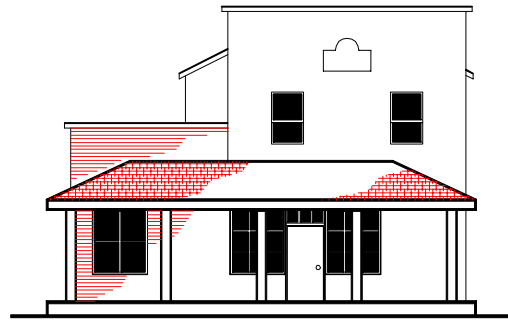
Desirable - false-front store front
